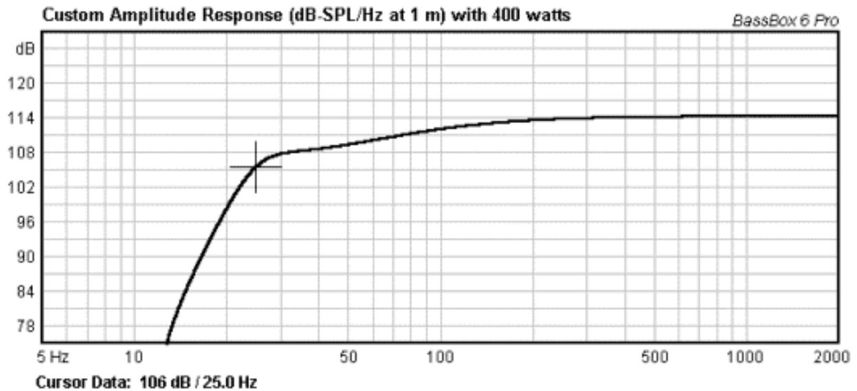
At 25 Hz the maximum is 106 dB, but we need to inspect the cone and slave excursion before proceeding with the design:
