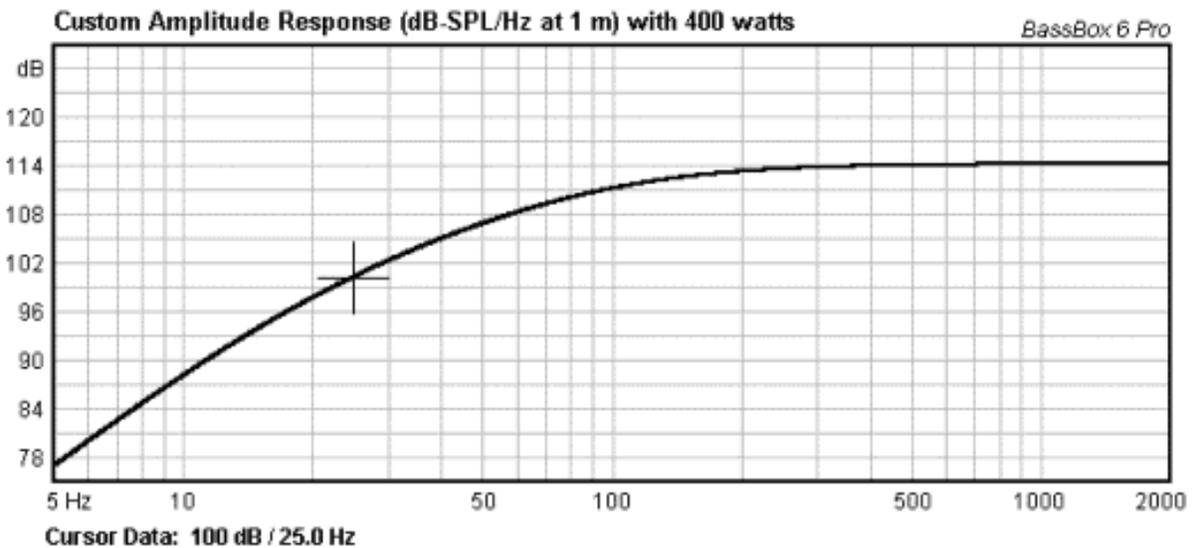
It can be seen that the maximum level at 25 Hz is only about 100 dB with 400W of amplifier power. This means that we will not be able to achieve our goal of minimum 105 dB SPL at 25 Hz without exceeding the maximum powerhandling of the driver further.
